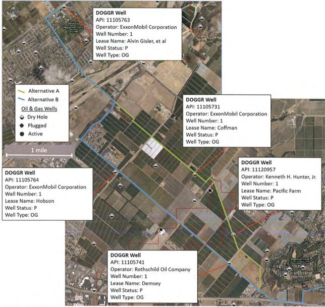
Figure 1. Annotated satellite image of the proposed water pipelines and oil and gas wells. The DOGGR well-record review includes wells proximal to proposed pipeline paths.
